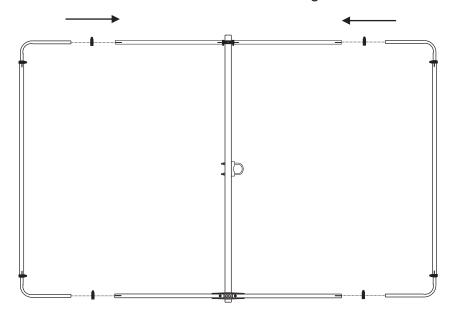
Attach the balun assembly to either of the insulators, it does not matter. Remove the nuts holding the tubes and use them to secure the brackets as shown. Use cable ties or electrical tape to secure the coax to the boom
