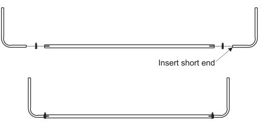
Slide a hose clamp over each short tube. Insert the side assemblys into the main section. Adjust the length of the side section so that it will slide into the short tubes easily. Snug the hose clamps so that the tubing does not move. Install the U-bolt into the boom using the hardware included
